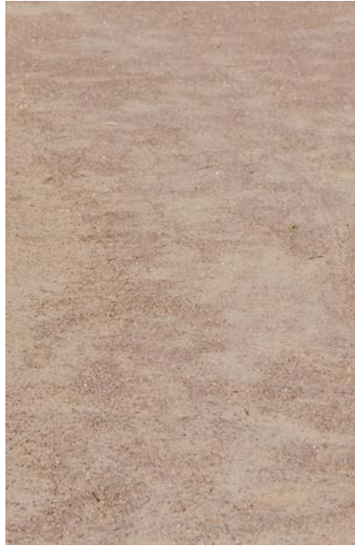
Stabilized soil Decomposed Granite
